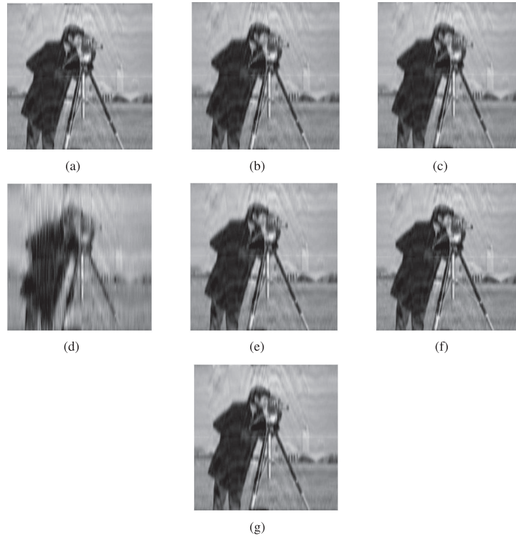
FIGURE 11. Deblurring image with other popular \beta . (a) \beta^{HS} , PSNR = 23.7595. (b) \beta^{FR} , PSNR = 23.1993. (c) \beta^{PRP} , PSNR = 23.1458. (d) \beta^{CD} , PSNR = 19.4664. (e) \beta^{LS} , PSNR = 23.0885. (f) \beta^{DY} , PSNR = 23.8327. (g) \beta^{HZ} , PSNR = 23.2477.
