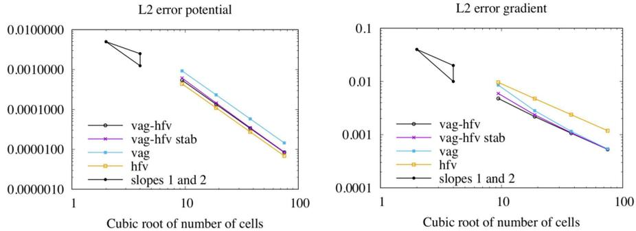
FIGURE 6. Convergence in  $L^2$  norm of the potential (*left*) and of the gradient (*right*) on the family of hybrid meshes (hexahedral and pyramidal cells) with anisotropic permeability and for the VAG, HFV, VAG–HFV and the stabilised VAG–HFV schemes.
