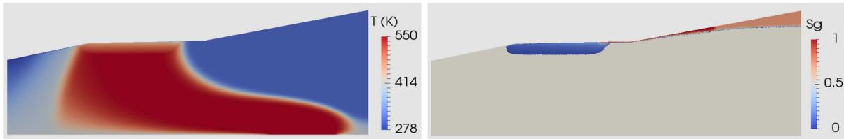
FIGURE 16. Reference temperature (in K) and gas saturation above the threshold of  $10^{-2}$  at final time (650 years) obtained with the refined Cartesian-triangle mesh combined with the VAG-TPFA scheme.
