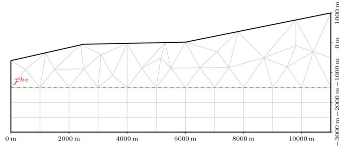
FIGURE 15. Coarse hybrid Cartesian-triangular mesh.
