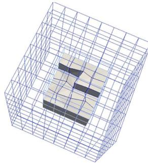
FIGURE 2. Hexahedral mesh obtained for  $N = 8$  and composed of cubic cells in the HFV subdomain  $\Omega \setminus \overline{\Omega}^v$  and of randomly perturbed cubic cells in the VAG subdomain  $\Omega^v = (0.25, 0.75)^3$ .
