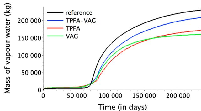
FIGURE 20. Mass of vapour water in the reservoir as a function of time for the various discretizations.
