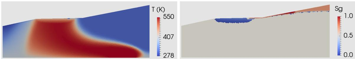
FIGURE 18. Temperature (in K) and gas saturation above the threshold of  $10^{-2}$  at final time (650 years) obtained with the TPFA scheme on the Voronoi mesh.
