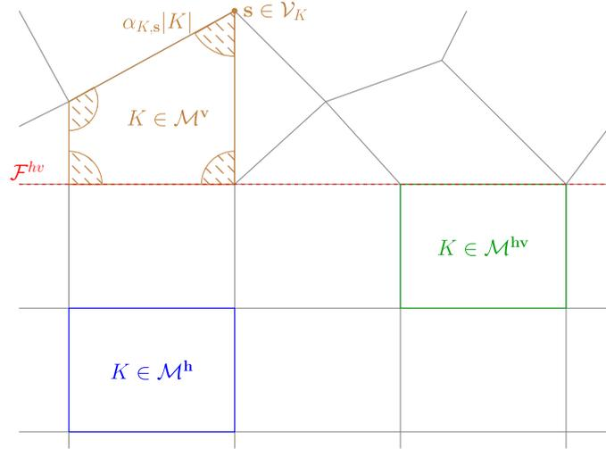
FIGURE 9. Illustration on a 2D mesh of the distribution of the volumes  $\alpha_{K,s}|K|$  to each node  $s \in \mathcal{V}_K$  of the cell  $K \in \mathcal{M}^v$  in the case of a single rock type.
