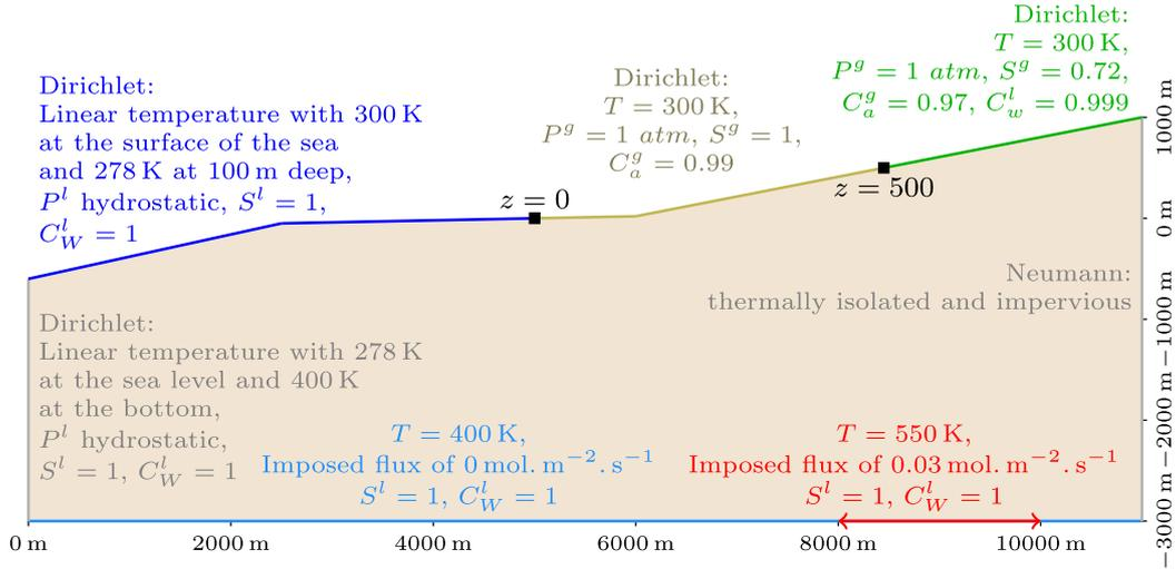
FIGURE 14. Illustration of the two dimensional geothermal reservoir and of the various conditions applied at its boundary.
