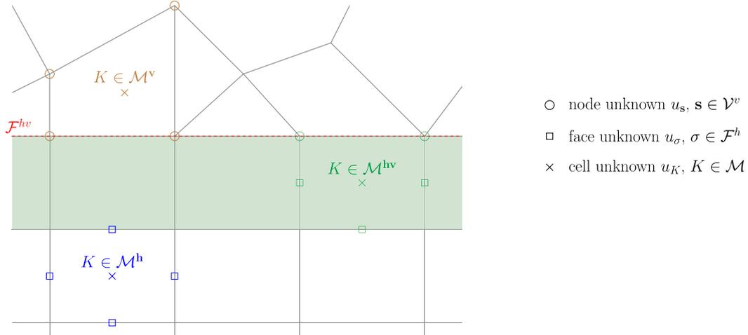
FIGURE 1. Illustration on a 2D mesh of the partition of the cells between the VAG cells  $K \in \mathcal{M}^v$ , the HFV cells  $K \in \mathcal{M}^h$  and the interface cells  $K \in \mathcal{M}^{hv}$ . Examples of cell (crosses), node (circles) and face (squares) degrees of freedom of  $\text{dof}_{\mathcal{D}}$  in the VAG, HFV and interface regions.
