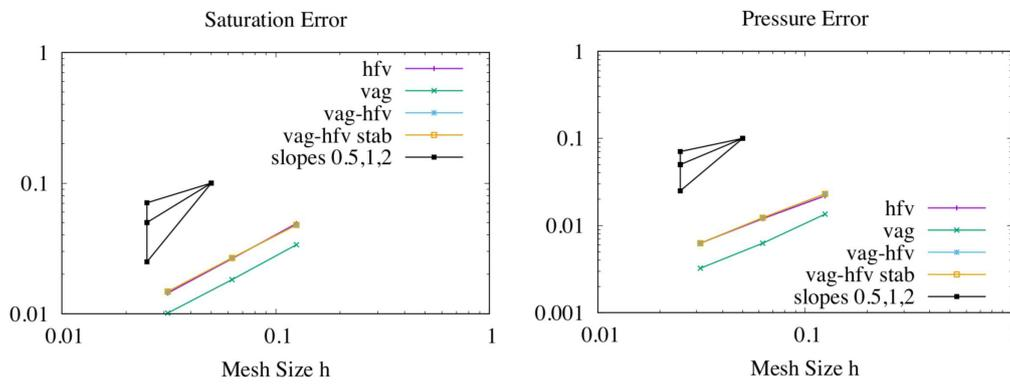
FIGURE 13. Convergence in space time discrete  $L^1$  norm of the saturation and the non-wetting pressure on the family of hybrid meshes and for the VAG, HFV, VAG–HFV and the stabilised VAG–HFV schemes.
