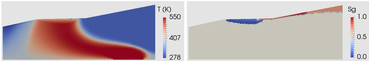
FIGURE 17. Temperature (in K) and gas saturation above the threshold of  $10^{-2}$  at final time (650 years) obtained with the VAG scheme on the triangular mesh.
