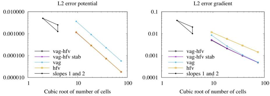
FIGURE 5. Convergence in  $L^2$  norm of the potential (*left*) and of the gradient (*right*) on the family of hybrid meshes and for the VAG, HFV, VAG–HFV and the stabilised VAG–HFV schemes.
