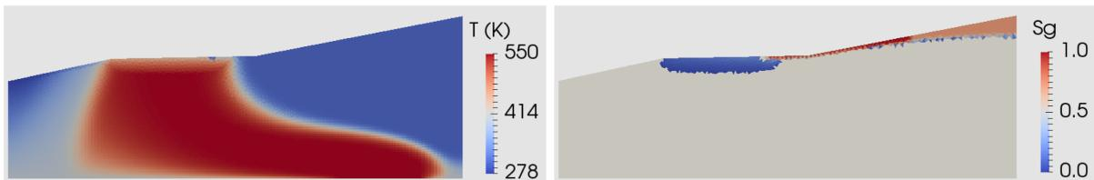
FIGURE 19. Temperature (in K) and gas saturation above the threshold of  $10^{-2}$  at final time (650 years) obtained with the VAG-TPFA scheme on the Cartesian-triangular mesh.
