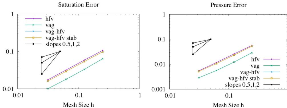
FIGURE 11. Convergence in space time discrete  $L^1$  norm of the saturation and the non-wetting pressure on the family of hexahedral meshes and for the VAG, HFV, VAG–HFV and the stabilised VAG–HFV schemes.
