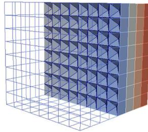
FIGURE 12. Hybrid mesh obtained for  $N = 8$  and composed of cubes in the HFV subdomain  $\Omega \setminus \overline{\Omega}^v$  and of pyramids in the VAG subdomain  $\Omega^v = (0.5, 1) \times (0, 1)^2$ .
