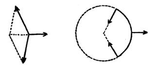
c) In one dimension, the force law and the torque law, its derivative, must give one sole condition : it follows that opposite forces applied to a solid line and parallel to it are in equilibrium.
