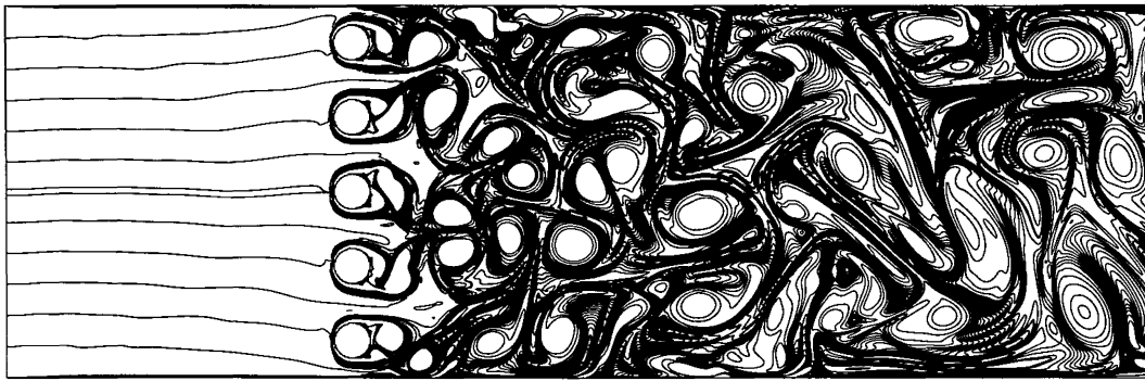
FIGURE 3. Vorticity contours at Re = 5 \times 10^5 .
