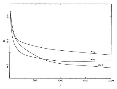
Fig. 7. – Time-dependence of the diffusion coefficient of the process  $y_t - y_0$ , computed along three different orbits. The quantity K, is defined as  $K = (y_T - y_0)/N$  represents the number of times the orbit has wrapped around the torus in the y-direction.
