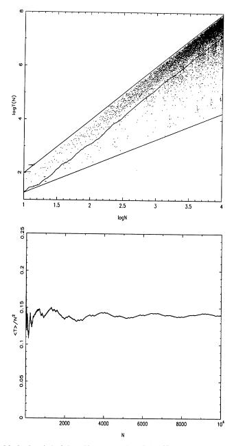
Fig. 6. – Maximal period of the orbits, on a lattice of size N, for the golden mean rotation number. *Top:* the period function T(N), with upper and lower envelopes, and its average order  $\langle T \rangle$ . *Bottom:* normalized average order  $\langle T(N) \rangle / N^2$ .
