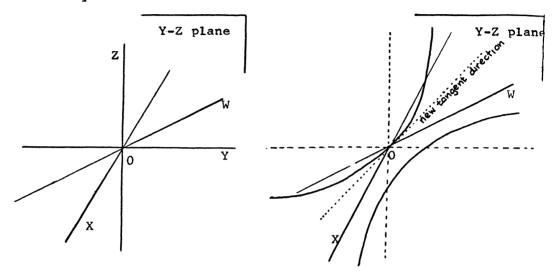
the Z and Y axes have deformed to a hyperbola through the origin with tangent direction depending on that of X and W
