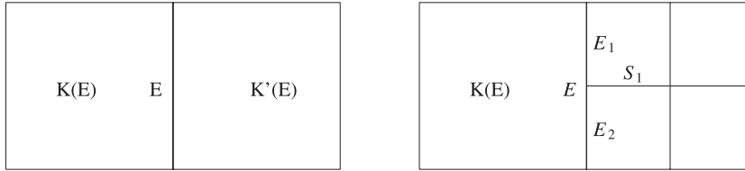
FIGURE 3. Two dimensional configuration for the case of a regular inner face i.e. E \in \mathcal{E}_r (left) and for the case of an irregular inner face i.e. E \in \mathcal{E}_i (right).
